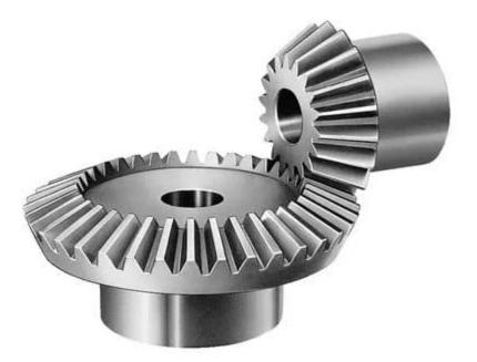
Bevel gears are not your standard cylindrical gears. They come on a conical surface that allows you to change the direction of the transmission on intersecting shafts. Generally, bevel gears work with  $90^0$  angles. However, you can use them on other configurations as well.
