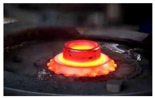
Theoretically, forging is an excellent gear manufacturing process for heavy-duty applications because of a simple reason. Forging requires heat treatment, which means that the resulting gear would have better fatigue properties. However, the tremendous force required for the forging process limits the size and thinness of this process.
