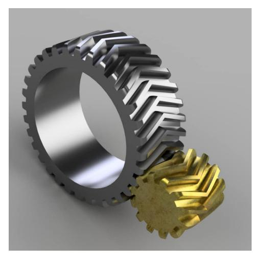
Most of the applications of helical gears are the same as spur gears. However, the angled teeth play a huge role in reducing the impact load and making the operations smoother. This means less noise as well but at the cost of efficiency. Relative to spur gears, a helical gear train will have more losses and will also need thrust bearings because of the shape.
